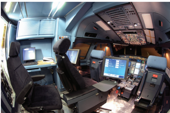
Instructor operator station (IOS) update completed
