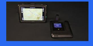
With CAE SkyDeploy's scalable moving map display, the aircrew can precisely follow the displayed search pattern and receive in-flight search pattern updates from the ground control center. The system has a built-in function for accurately marking the location of wildfires or smoke and menu-driven reports are automatically transmitted via Satcom to the ground control center.
