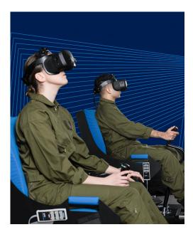
Visual immersion is enabled via a headset with high-resolution out-the-window visuals generated by the CAE image generator and delivering the visual acuity to read the instrument panel. Physical controls may include generic or replicated cockpit controls and instrumentation for realistic to true-to-life sensory feedback.
