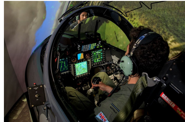
One of the RAAF’s student pilots flies a Hawk Mk127 simulator at RAAF Base Williamtown during a trial of eye-tracking technology.
