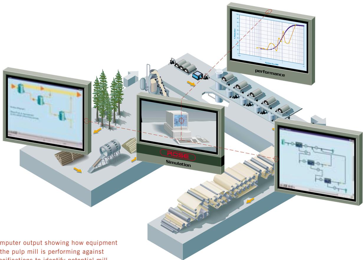
Computer output showing how equipment in the pulp mill is performing against specifications to identify potential mill deficiencies and improvement options
