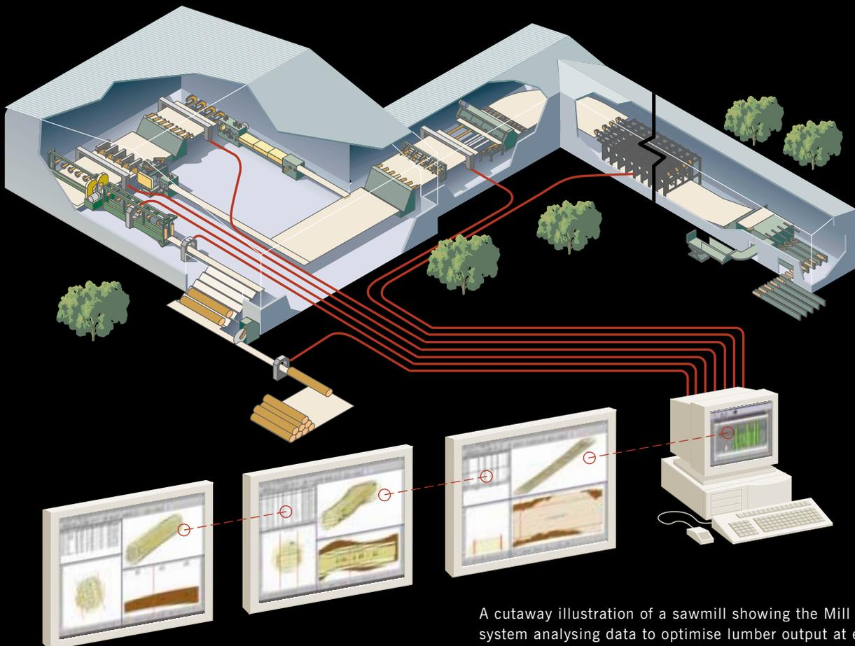
A cutaway illustration of a sawmill showing the Mill Host system analysing data to optimise lumber output at each stage of the mill operation
