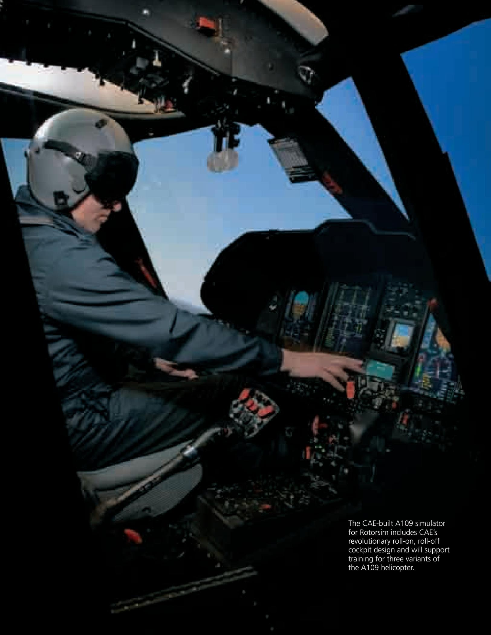
The CAE-built A109 simulator for Rotorsim includes CAE's revolutionary roll-on, roll-off cockpit design and will support training for three variants of the A109 helicopter.
