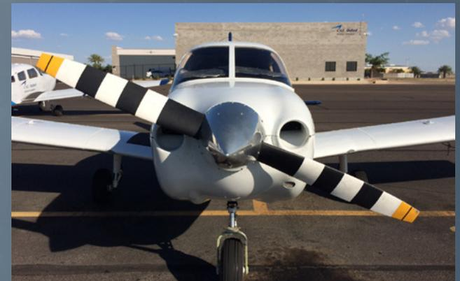
By adding black lines on the propellers, concentric circles are visible when propellers are in motion.
