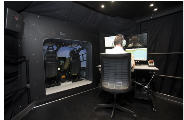
The new CAE 700MR flight training device features a spacious cockpit interior for instructors and rear-crew training as shown in the H135 FTD for the UK MFTS program.
