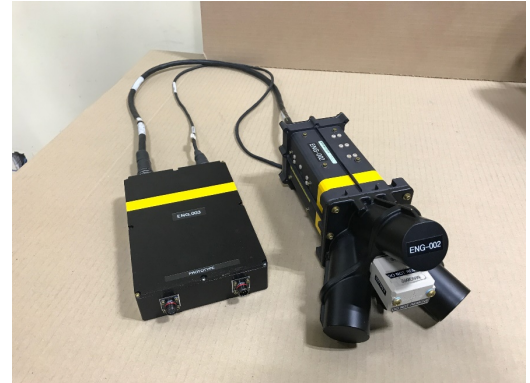
CAE MAD-XR is significantly more compact than previous MAD systems which allows it to be extended to platforms such as helicopters, unmanned aerial vehicles and small fixed-wing aircraft
