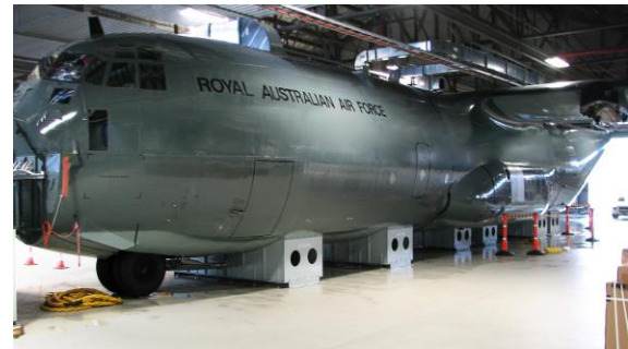
The new C-130J Fuselage Trainer for the Royal Australian Air Force at Richmond will provide a safe, cost-effective and realistic training environment for loadmasters and rear crew.
