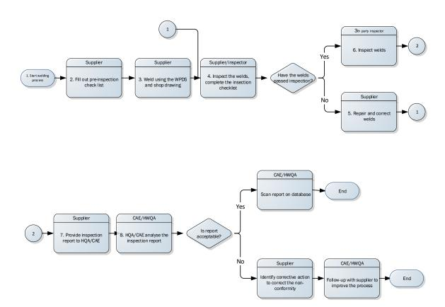
Supplier must control the welding process and complete required inspections prior to start of welding, during welding and after welding process.
