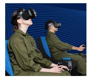
Visual immersion is enabled via a headset with high-resolution out-the-window visuals generated by the CAE image generator and delivering the visual acuity to read the instrument panel. Physical controls may include generic or replicated cockpit controls and instrumentation for realistic to true-to-life sensory feedback.
