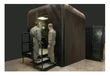
Each high-fidelity OFT cockpit is mounted on a 3 degree-of-freedom (DOF) vibration platform. The vibration platform is mounted on a 6-DOF electric motion system. A 200 degree horizontal x 45 degree vertical visual display, supplemented with pilot and co-pilot chin windows, supports out-the window imagery.
