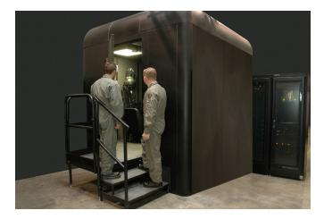
Each high-fidelity OFT cockpit is mounted on a 3 degree-of-freedom (DOF) vibration platform. The vibration platform is mounted on a 6-DOF electric motion system. A 200 degree horizontal x 45 degree vertical visual display, supplemented with pilot and co-pilot chin windows, supports out-the window imagery.
