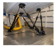
An alternative is to completely replace the hydraulic motion system with a new electric motion system that will require less maintenance, less refurbishments, and save energy.
