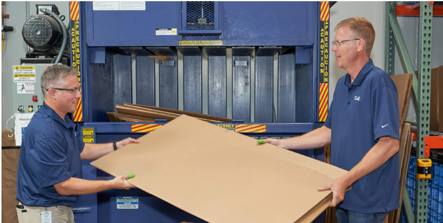
CAE Healthcare employees load boxes into an on-site baler for more efficient recycling.
