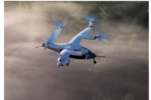
The all-electric Joby aircraft in flight above the company's Electric Flight Base in California
