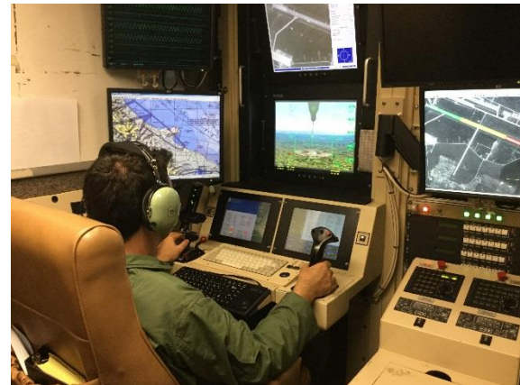
The Predator Mission Trainer developed by CAE and GA-ASI for the Italian Air Force is capable of delivering zero flight time training.
