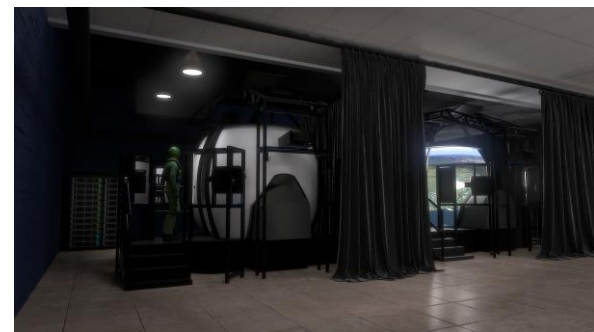
The CAE Medallion MR e-Series Visual System is designed for interoperability and networking to support training tasks such as formation flying and aerial refueling
