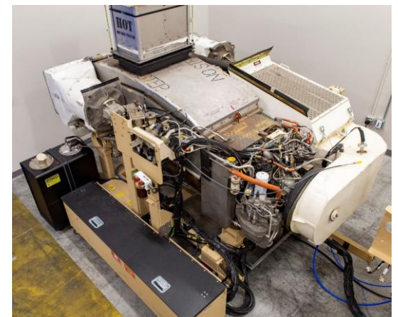
The Abrams engine maintenance trainer will support diagnostic and troubleshooting maintenance training tasks.
